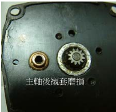
Motor Gear & Bushing damaged
