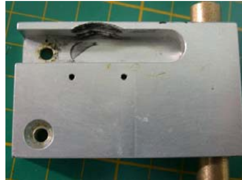
Slip Plate Damaged
