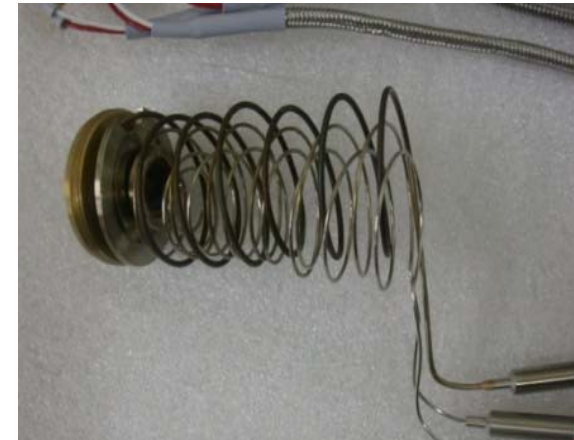
Internal Heater & T/C
