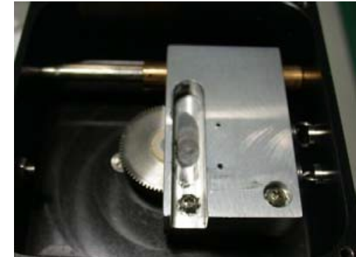
Slip Plate Damaged
